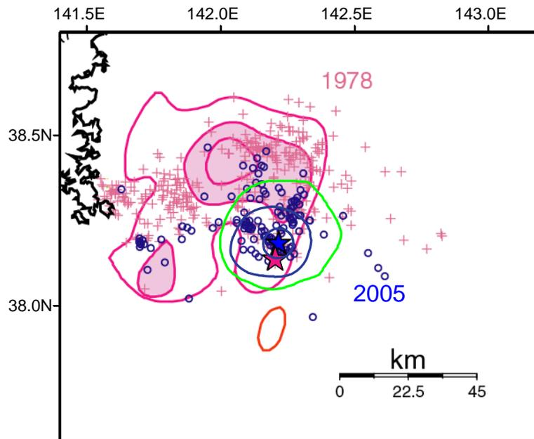
Fig. 4 Comparison of the coseismic slip distributions of the 2005 Miyagi-Oki earthquake estimated by seismic waveform inversion (blue contours) performed by Yaginuma et al. (this issue) and the geodetic inversion using GPS data in this study (green contours) with an interval of 0.3 m. Blue circles and red crosses indicate epicenters of aftershocks for 2 days of the 2005 and 1978 events, respectively, relocated by Okada et al. (2005).
