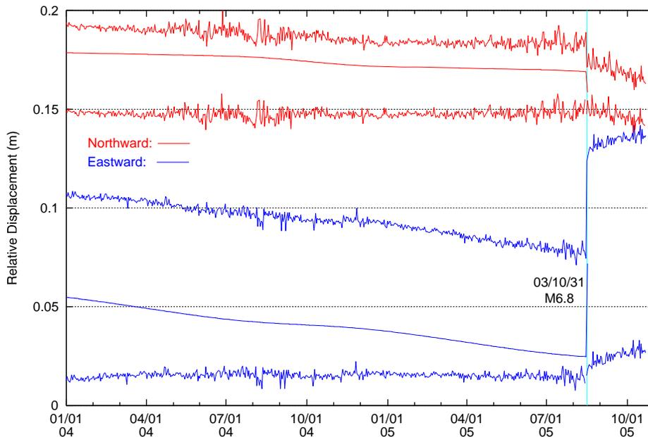
Fig.2 Example showing how to evaluate postseismic displacements at a GEONET station, 0550 (Ayukawa). Red and blue traces denote northward and eastward displacements, respectively. Top, middle, and bottom of each component represent raw data, linear trends with annual and semi-annual variations and coseismic step estimated by least square fitting, and residuals, respectively.
