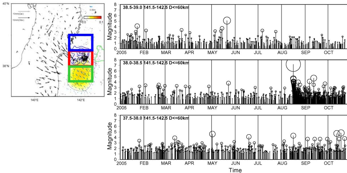
Fig. 5 Magnitude-Time diagrams in the three areas in and around the aftershock area of the 2005 earthquake. Top, middle, and bottom panel represent the northern neighborhood of the aftershock area, the aftershock area, and its southern neighborhood, respectively. They are shown by blue, red, and green rectangles in the insert map.
